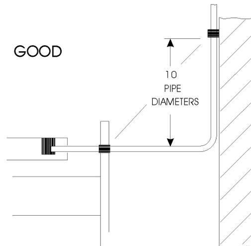
3. DON'T OVER SUPPORT PIPING when it is attached to the compressor rack. It must be free to float without stress.
