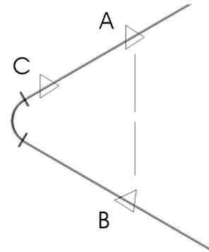
2. CORNERS MUST BE SUPPORTED and cannot be left free to pivot around the A-B axis as shown above.
